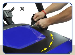
If any air bubbles remain, use a razor blade tip to slightly puncture, then smooth over with Squeegee (03-043).
